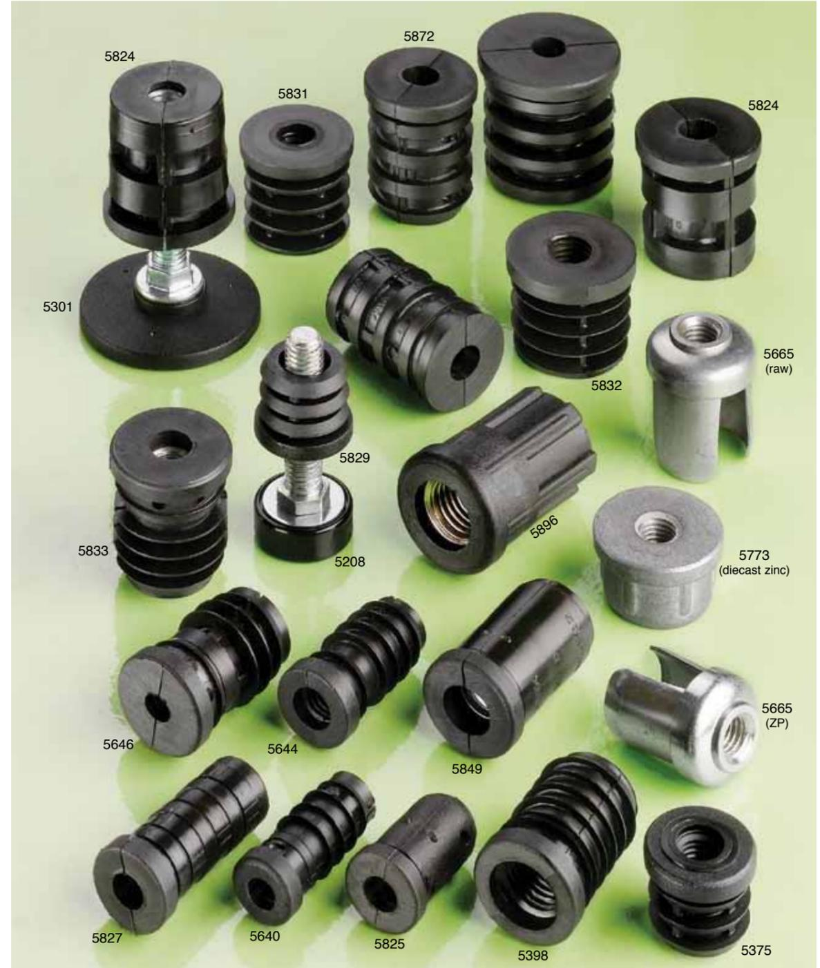
**Expanders use the "Rawplug" effect.** Expander inserts are made of 2 matching moulded Nylon pieces with 2 hex nuts sitting inside the tapered conical cavities. Tightening a threaded bolt or screw into the Expander for attaching a castor to a round tube presses the hex nuts downward, making the outer walls of the insert move sideways tightly gripping the inner wall of the tube, this is known as the "Rawplug" effect.
